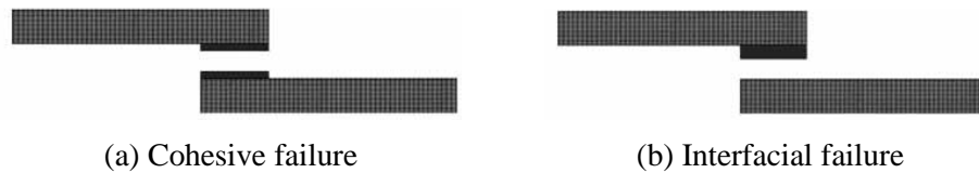
Figure 4. Failure modes of adhesive joints.
