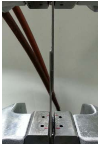
Figure 2. Specimen of dissimilar metal bond joint; overlap length: 20 mm, 40 mm, and 60 mm.
