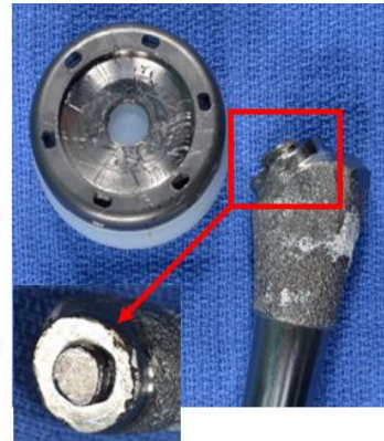
Fig. 8 (right) Humeral tray/polyethylene cup component and Morse taper retained within humeral stem. Note smooth edges of fracture site.
