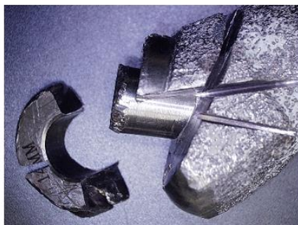
Fig. 9 Result of the removal of the embedded taper using a rotary tool. Every effort was made to ensure no damage was inflicted on the taper during removal.
