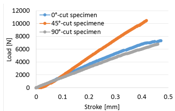
Figure 4. Load-stroke for SMC specimens along 0°, 45° and 90° directions
