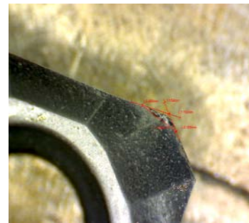
(b) Measurement of tool wear region
