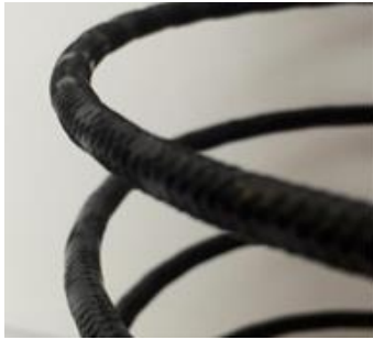
Figure 5. Resin impregnated braided BFRP.
