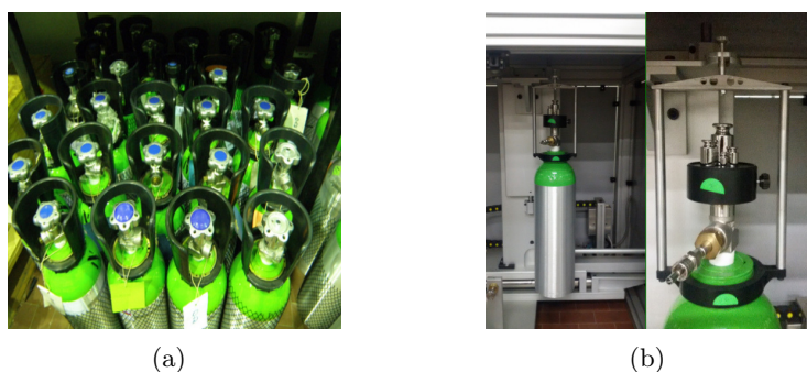
Figure 1. a) Primary gravimetric gas mixtures produced at INRiM; b) Detail of the INRiM facility for the weighing of a primary gas mixture, with calibrated mass standards.
