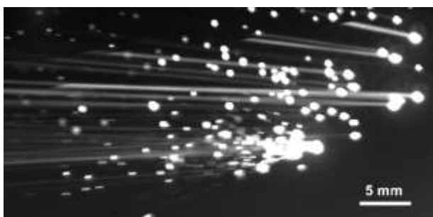
Figure 1. Group of tungsten droplets being a source of high-velocity emissions. Scale 51.9 microns/ pixel, frame exposure time is 10 \mu s.
