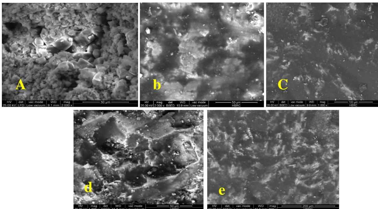
**Figure.1.** Shows the SEM micrographs of (A) untreated sample, (b). Sample treated with Pure Paraloid – B72, (c). Sample treated with Ca (OH) <sub>2</sub> /polymer nanocomposites, (d). Sample treated with Paraloid – B72 after thermal aging and (e). Sample treated with Ca (OH) <sub>2</sub> /polymer nanocomposites after thermal aging.
