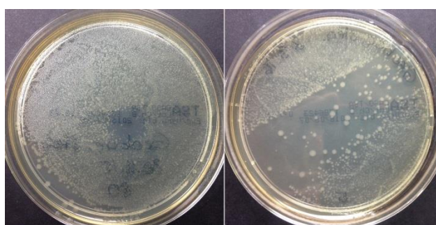
Figure 7. Comparison of results after 60 s of treatment. Left: non-thermal plasma (PB3), dish pre-incubated after plating for 6h at 56°C. Right: thermal plasma (LARGE), direct treatment of endospores
