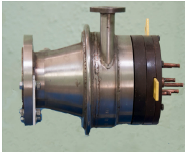
Figure 1(b) Photograph of three-phase electric arc plasma torch.
