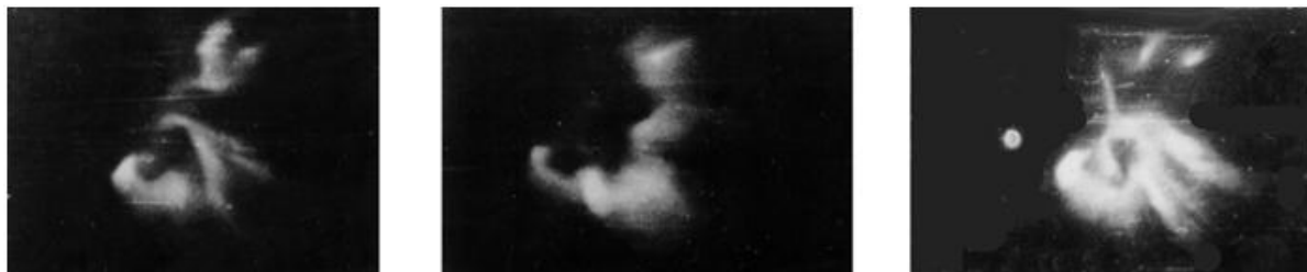
Figure 4. Frames of reswitching of arcs in the plasma torch chamber at atmospheric pressure (root mean square value of arc current – 200A, working gas flow rate – 24 g/s )
