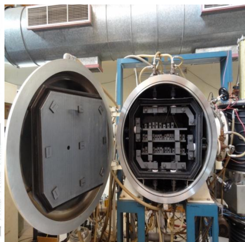
Figure 2. Vacuum Furnace loaded with graphite tiles.
