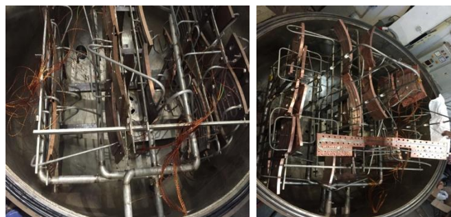
Figure 8. Baking facility for PFC modules, and Header pipe, isolators and bellows.
