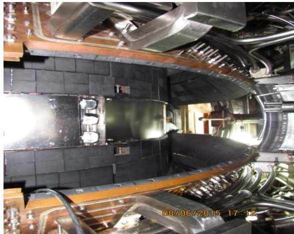
Figure 11. Final assembly of PFC modules in SST-1 main vessel.
