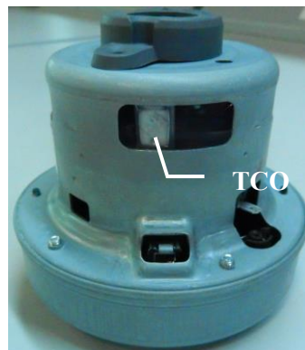
Figure 3. TCO inside a universal motor.
