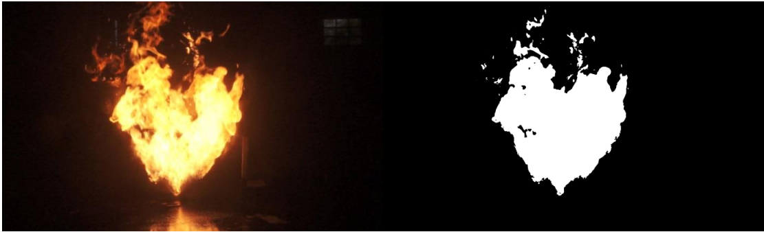
Figure 4. Flame area (indicated by the white area) of an image from Fractal 1 at equivalence ratio 1.0
