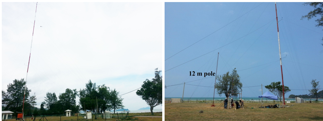
(a) The weather station infrastructure, EKOMAR (b) EKOMAR snapshot taken approximately from the South, showing the South China Sea. snapshot taken from the West, showing the 12 m pole. The 60 m pole to the right was also utilized, but not discussed here. An intermediary pole in between the two (not clear) was used for the 3 m position.
