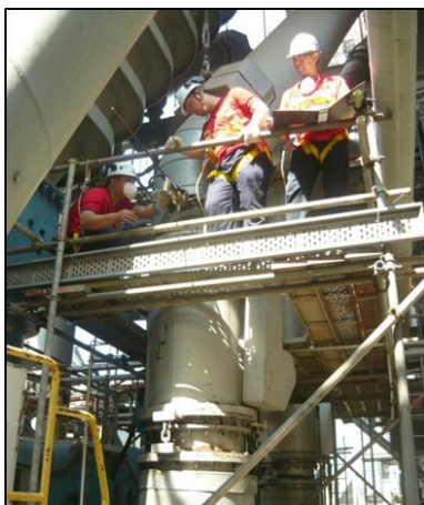
Figure 1: PC pipes velocity measurement by using Dirty Air Pitot
