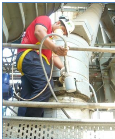
Figure 2: Pulverizer Fuel Sampler - extract coal sample
