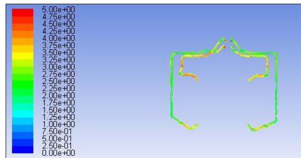
Figure 13. Contours of wall shear stress of mill 7 at coal particle size of 70 microns
