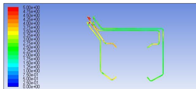
Figure 8. Contours of wall shear stress of mill10 at coal particle size of 100microns
