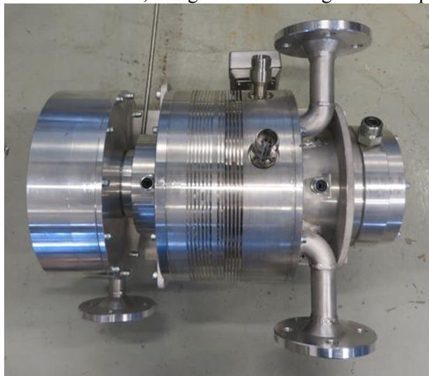
Figure 5. Turbogenerator. The turbine is located on the left, generator in the middle and pump on the right.
