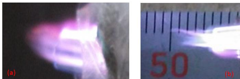
Figure 4. (a) Picture of plasma in Helium and (b) plasma discharge with Argon gas.
