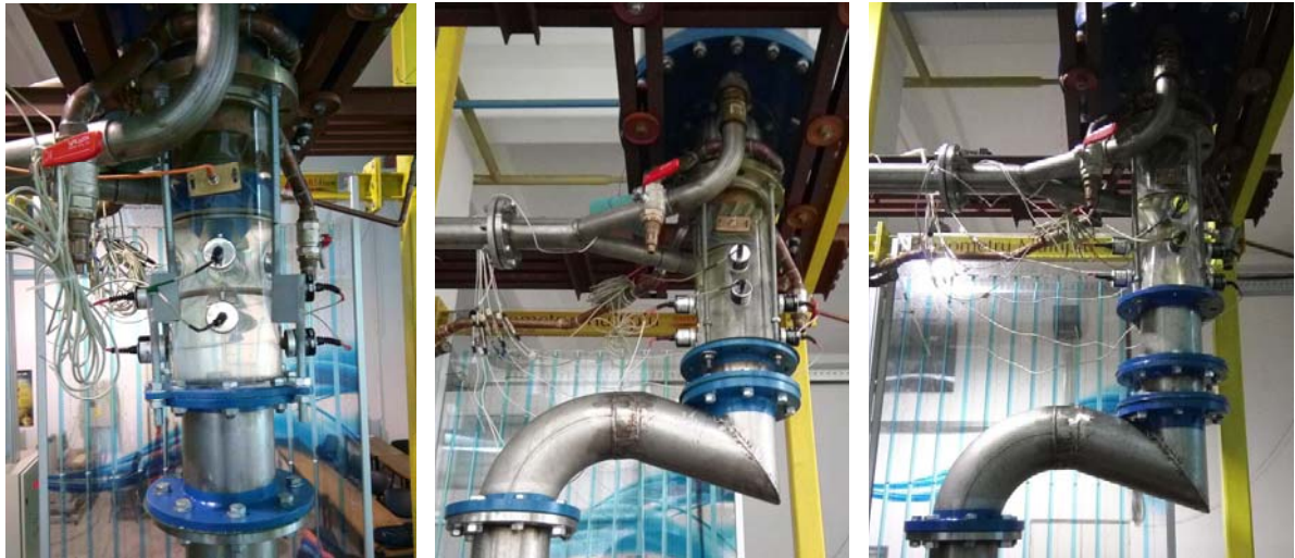
Fig. 2 Photo of the swirling flow test section considering three geometrical configurations: straight (S) and 74° sharp heel elbow together with pipe extensions of 0.1 m (HE74E01) and 0.3 m (HE74E03), respectively
