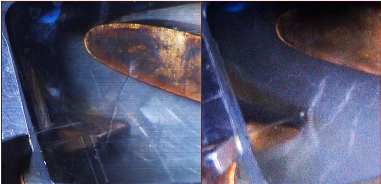
Figure 2. Cavitating vortices in the distributor
