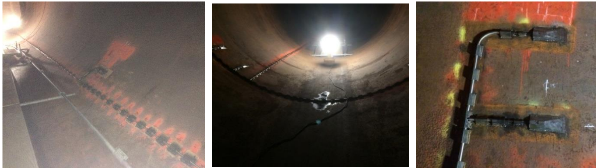
Figure 3: View of the pressure sensors installation in the penstock and spiral casing.
