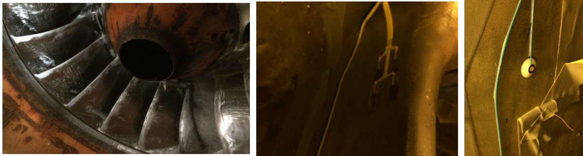
Figure 2. View of the cone of the runner where the telemetry system was installed and view of some strain gauges and pressure sensors located in the runner.
