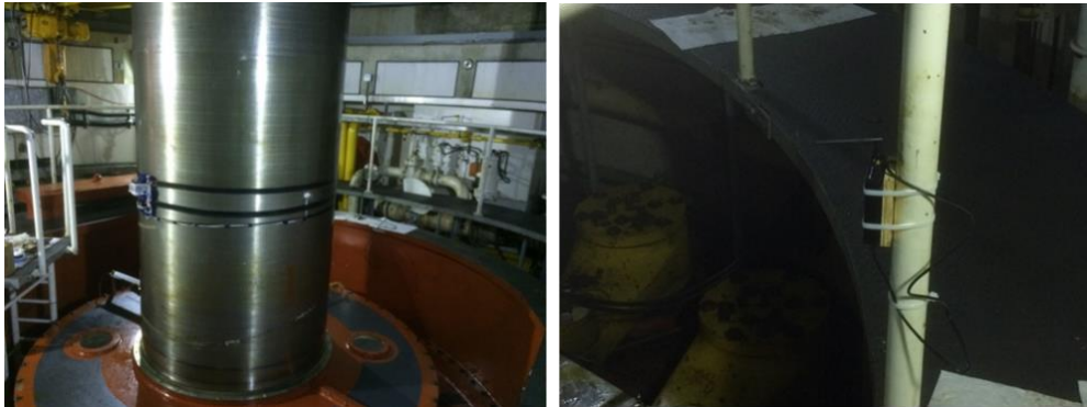
Figure 5. Telemetry system installed on the shaft for torque measurement.
