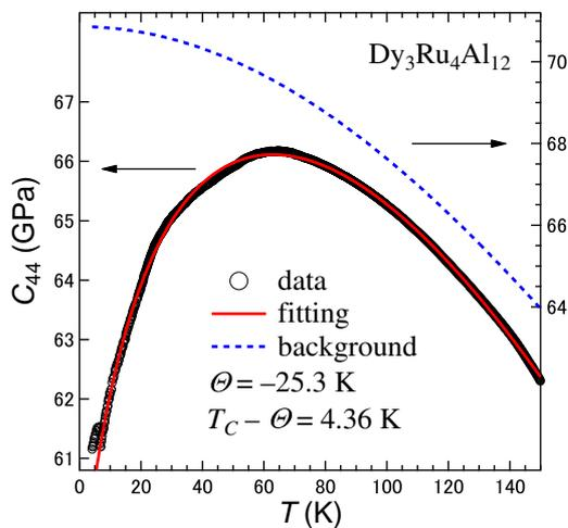
**Figure 3.** Temperature dependence of  $C_{44}$ . The red solid and blue broken curves demonstrate the fitting result and the background stiffness, respectively.
