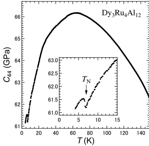
**Figure 2.** Temperature dependence of the transverse elastic modulus  $C_{44}$ . The inset represents the same data in an expanded scale below 15 K.
