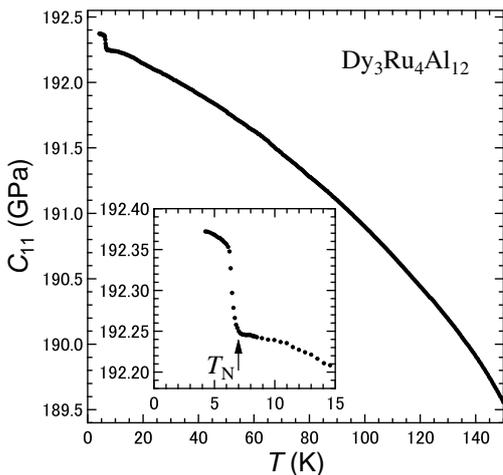
**Figure 1.** Temperature dependence of the longitudinal elastic modulus  $C_{11}$ . The inset represents the same data in an expanded scale below 15 K.
