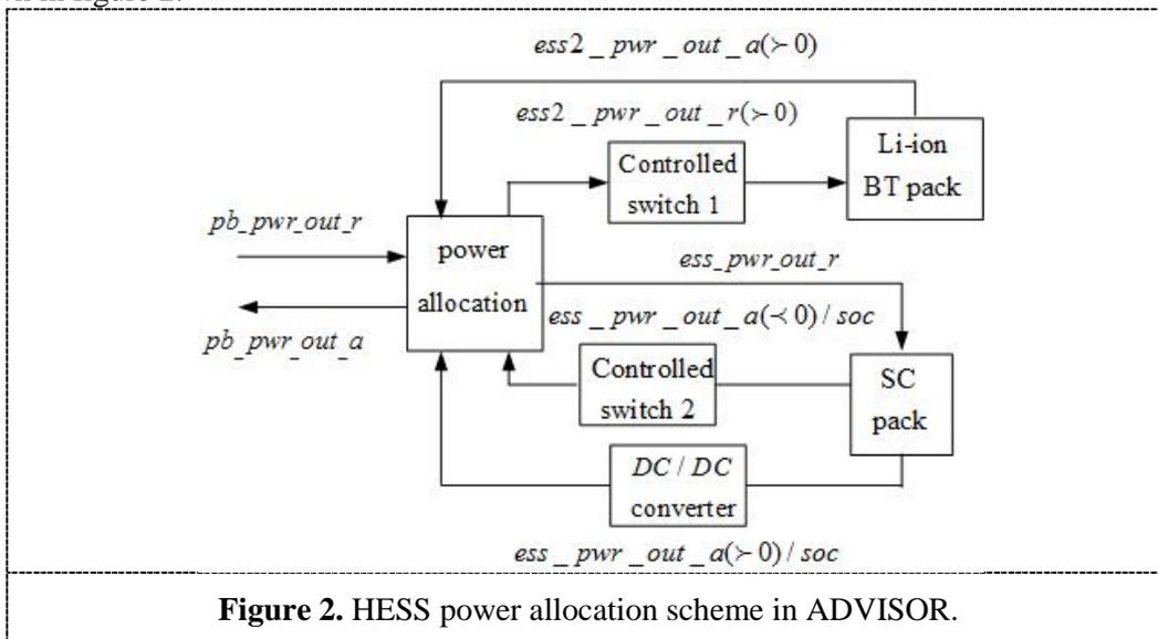
**Figure 2.** HESS power allocation scheme in ADVISOR.
