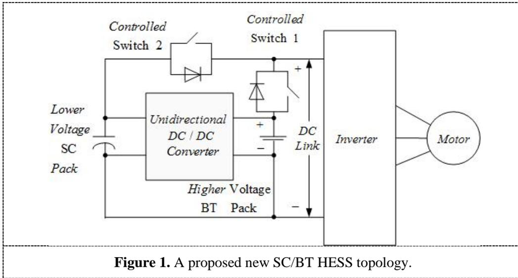
**Figure 1.** A proposed new SC/BT HESS topology.
