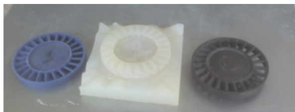
Figure 7. Creating a metal impeller for the micro-turbine engine (left to right): wax, a silicone mold, a metal casting.
