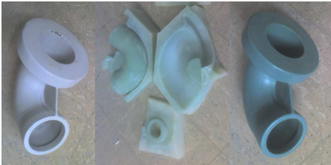
Figure 6. Creating a flue for the rocket engine (top to bottom): the master model, silicon mold, the wax metal casting.
