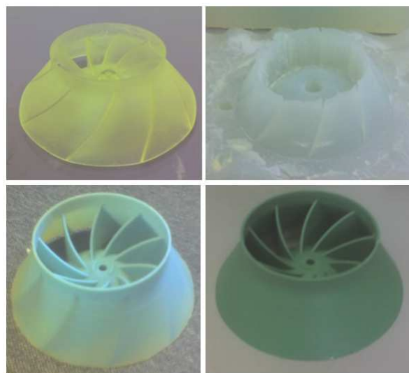
Figure 5. The steps of manufacturing the impeller: a stereolithography prototype, made of silicone mold, a cast in silicone stencil (for further casting metal, the cast in the sand mold is made of metal from parts.
