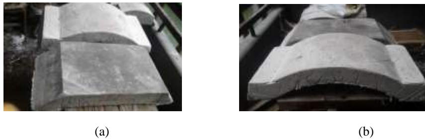
Figure 3. Conduit covers (a) flat cover (type 1) (b) curvy cover (type 2)
