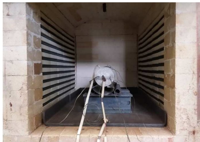
Fig. 3 – Sample positioning in the oven before the closure of tailgate of the oven.
