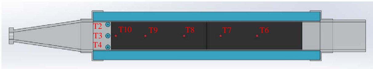
Figure 2. Temperature probes, test section.
