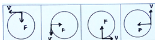
Figure 7. Linier velocity and centripetal force after circle share
