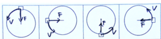
Figure 6. Linier velocity and centripetal force before circle share
