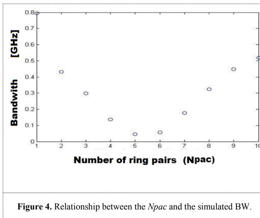
A symmetrical pattern can be appreciated indicating that the same BW can be achieved for different  $N_{pac}$ . This also implies that a greater  $N_{pac}$  is necessary to obtain a high BW, in the frequency of interest for electric field sensing.
