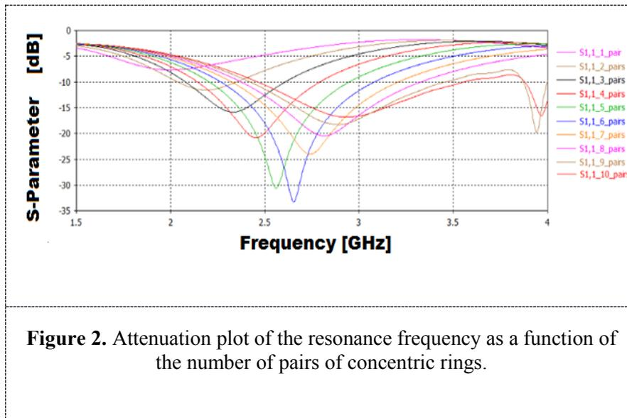
From the Figure 2 data, it was obtained the S11 parameter, the bandwidth (BW) at 3 dB and summarized in Table 2. The dependence of the number of concentric ring pairs on the resonance frequency was plotted in Figure 3. Additionally, a plot of number of pairs of concentric rings vs. bandwidth is shown in Figure 4.
