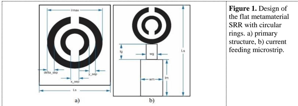
**Figure 1.** Design of the flat metamaterial SRR with circular rings. a) primary structure, b) current feeding microstrip.
