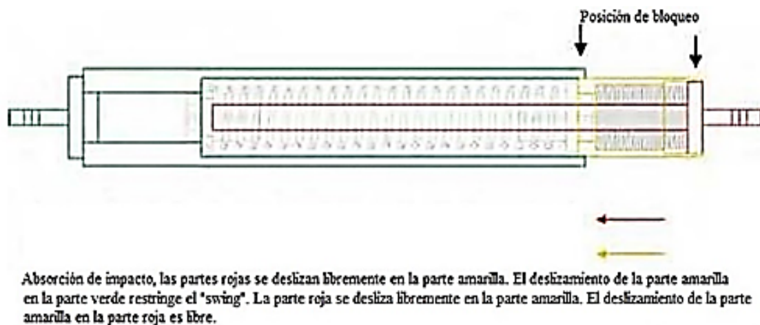
Figure 2. Linear actuator for balancing knee joint
