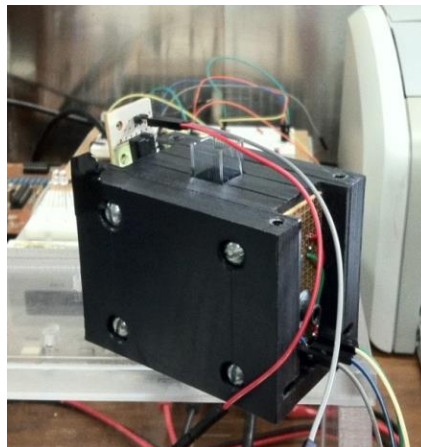
Figure 3. Detector cell and the emission source integrated
