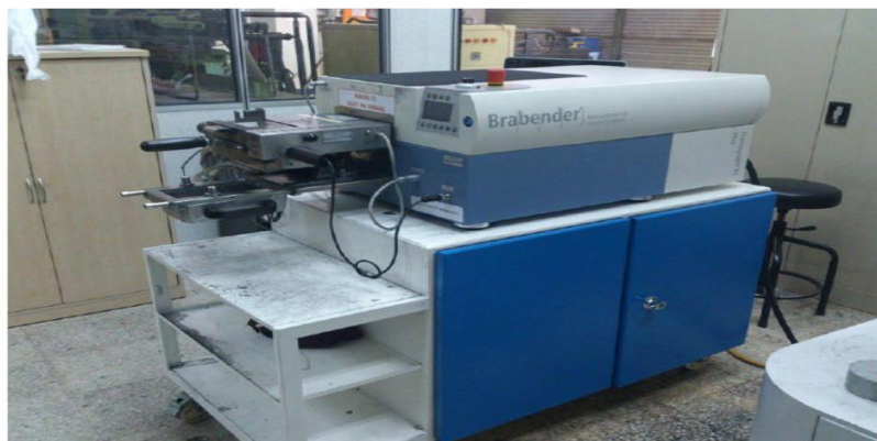
Figure 3. Compounding of Cu-Graphene using Brabender
