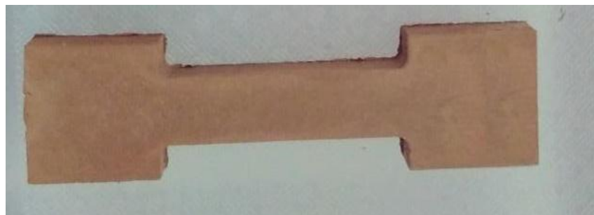
Figure 7. Physically defects free Cu-GNPs composite parts produced via PIM
