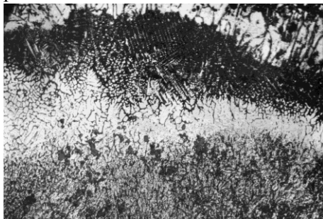
Fig. 3. A micrograph of ferrite Welding & Steel 40, x500
