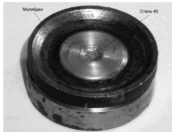
Fig. 5. Photo weldment of molybdenum and steel 40.
