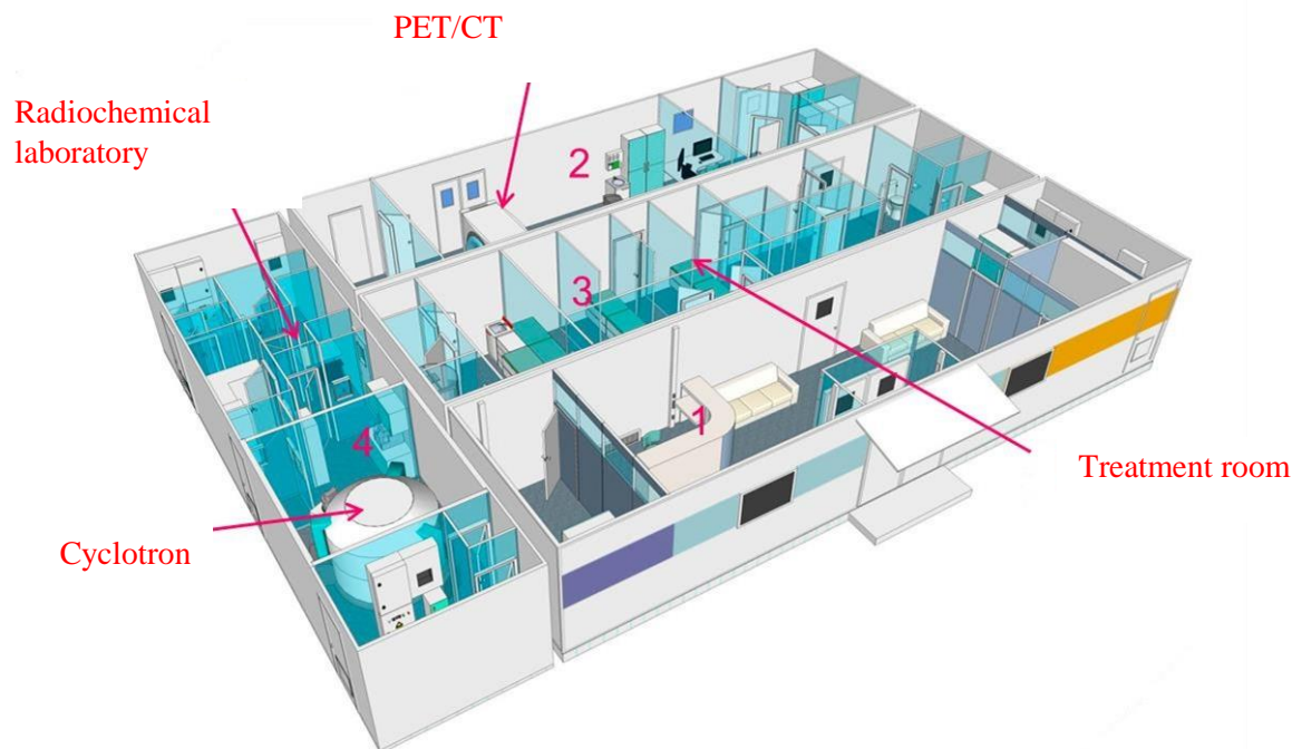
Figure 1. Mobile PET station diagram.
