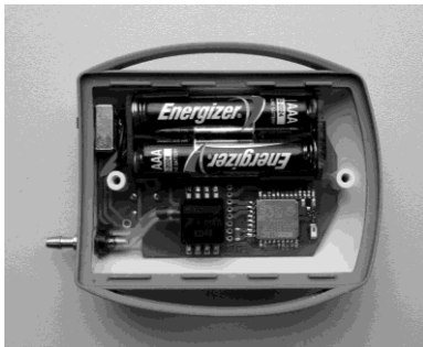
Figure 2. Internal placement of the WPS components.
