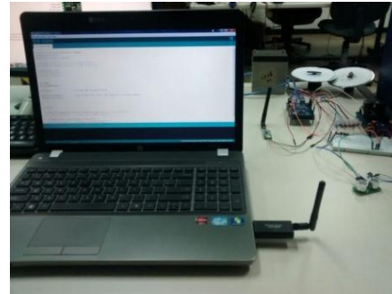
Figure 4. Functional test of wireless monitoring system
