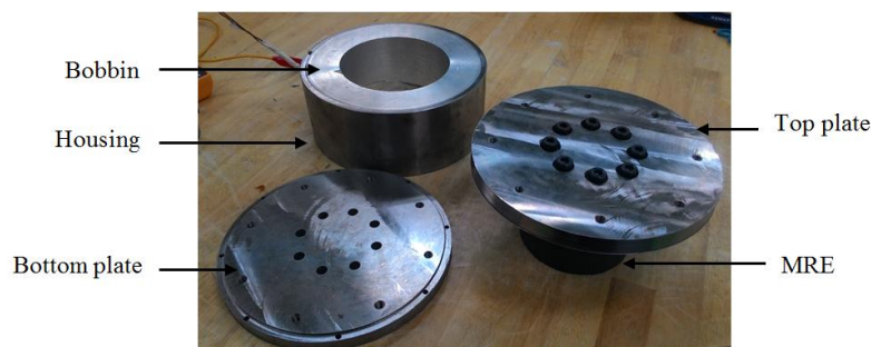
Figure 2. Main parts consist in a laminated MRE isolator
