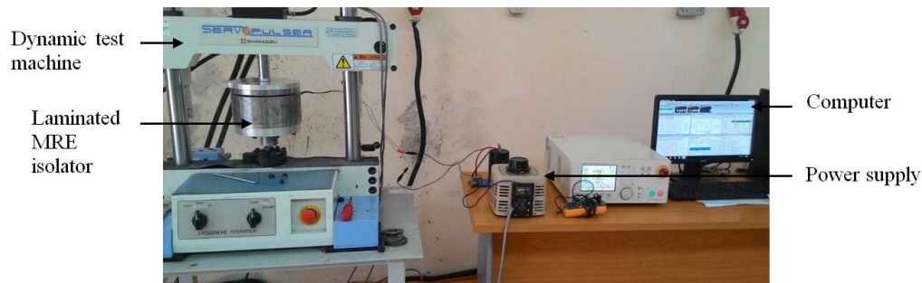
Figure 3. Experimental setups for laminated MRE isolator
