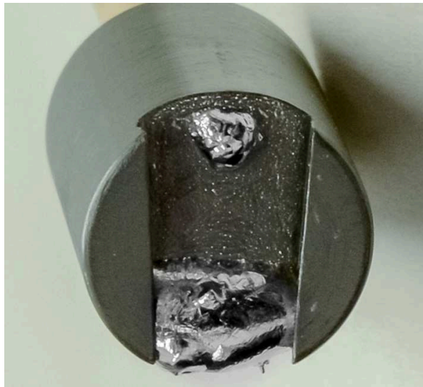
Figure 4. Frozen molten silver at sample 1.
