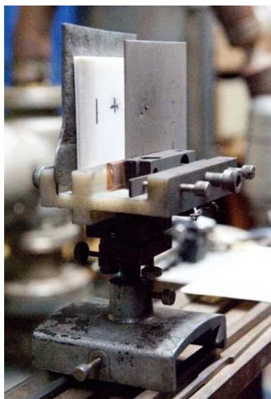
Figure 12. The photos of the target consisting of duralumin plate of 2 mm thickness, fluoroplastic plate of 8 mm thickness and lead plate of 3 mm.
