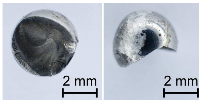
Figure 9. The photos of steel projectile 4 mm in diameter after the ballistic test.
