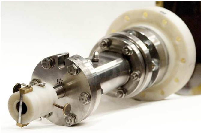
Figure 5. The photo of the barrel nozzle with a thin wire and a strip of copper foil.
