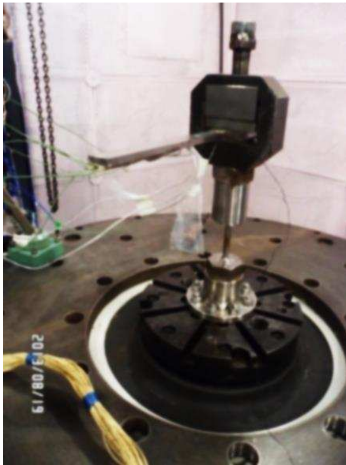
Figure 8. The gear for the thermal conductivity investigations of the materials in the field of vibration accelerations.
