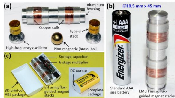
Figure 4. Photographs of the (a) harvester components before assembling, (b) assembled prototype alongside a standard AAA battery, and (c) complete package including multiplier and rectifier circuit for AC to DC conversion.
