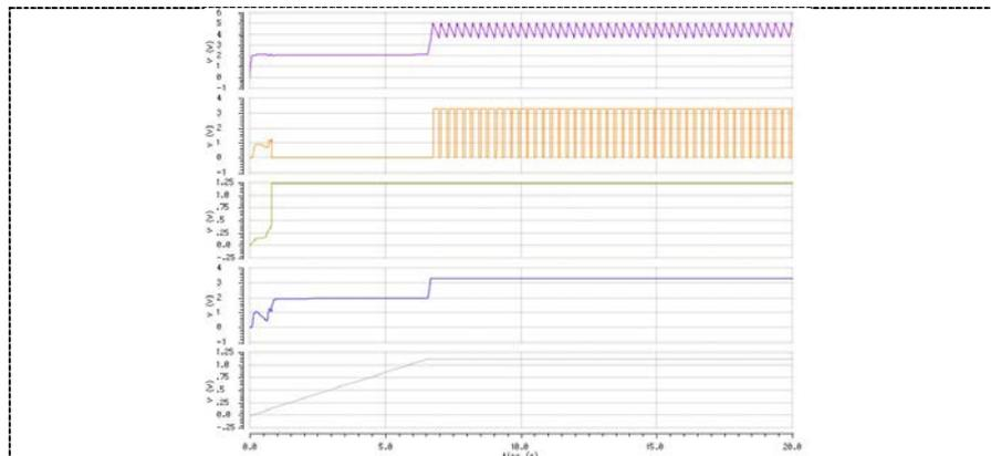
**Figure 5.** Caption of the transient simulation, from the ASIC1 extracted view, of the GATE control signal. Generation of the scenario operating phases. From the Top view to the bottom caption: (Top) Start-Up and harvest/measuring phases; VGATE signal that control the phases; Bandgap reference voltage; 3V3 LDO regulated voltage; (bottom) 1V1 LDO regulated voltage.
