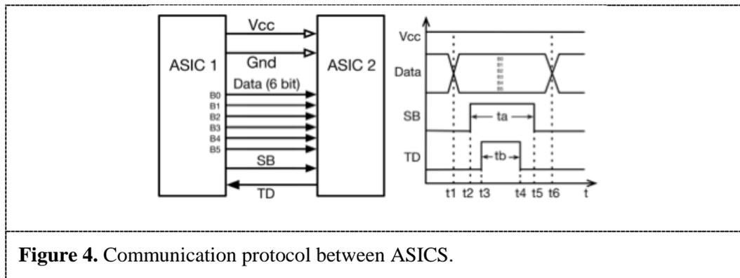
**Figure 4.** Communication protocol between ASICs.
