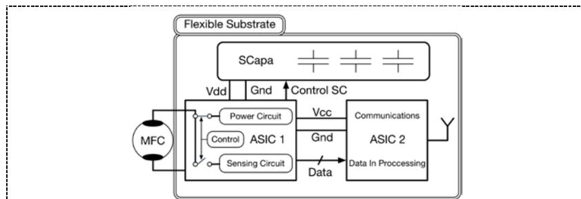
**Figure 1.** Main blocs for the Smarter Device.
