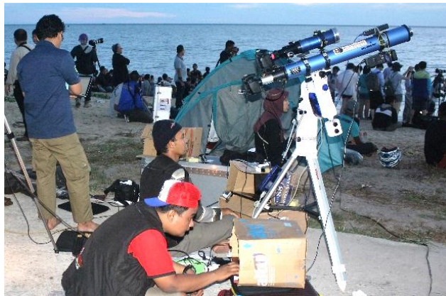
Figure 1. The ASEP controlled by three persons, the first person controlled the Mounting Vixen Spinx and SkyWatcher 910mm + Canon 60D, the second person controlled William Optics + Nikon D3300 and SQM, and the third person controlled Sony HCR MC5 and release-installing the Filter ND5.
