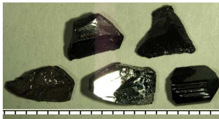
Figure 1. Photograph of BaFe 12-x Al x O 19 single crystals obtained from flux with mm-scale. One segment of the ruler corresponds to one millimetre.
