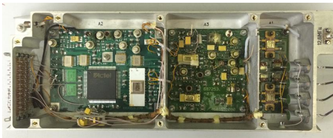
Figure 2. A new block of the microwave generator circuit.
