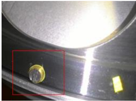
Figure 2. The mechanical method of the flywheel balancing.
