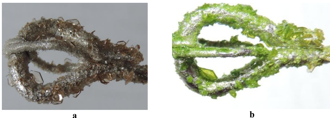
Figure 1. The seed holder with almost transparent \text{GaBO}_3 single crystals (a), and green online film of \text{FeBO}_3 on the \text{GaBO}_3 substrate (b).
