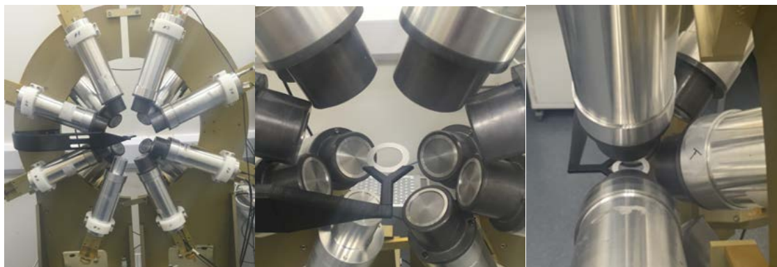
Figure 1 The NANA gamma-ray spectrometer at the UK National Physical Laboratory, comprising twelve individual \text{LaBr}_3(\text{Ce}) gamma-ray detector modules.
