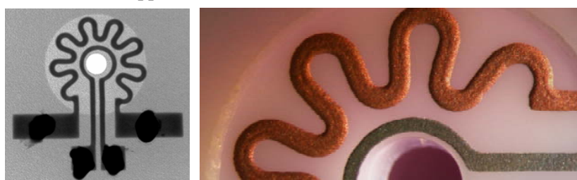
Figure 3. X-ray image of full-fledged combustor with a combined heater and oxygen supply meandering around the circular temperature sensor, inside which the sample inlet and gas outlet combine to make a bright circle (left), and microscope close-up of open reactor just after copper plating of the heater, not having affected the platinum temperature sensor (right).
